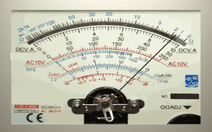
In the next slide, you will see the selector switch in the X10 position and then you will see a measurement of 15 Ohms on the meter. What is the actual resistance which is being measured? Note: Remember; the selector switch is in the X10 or times 10 position.
