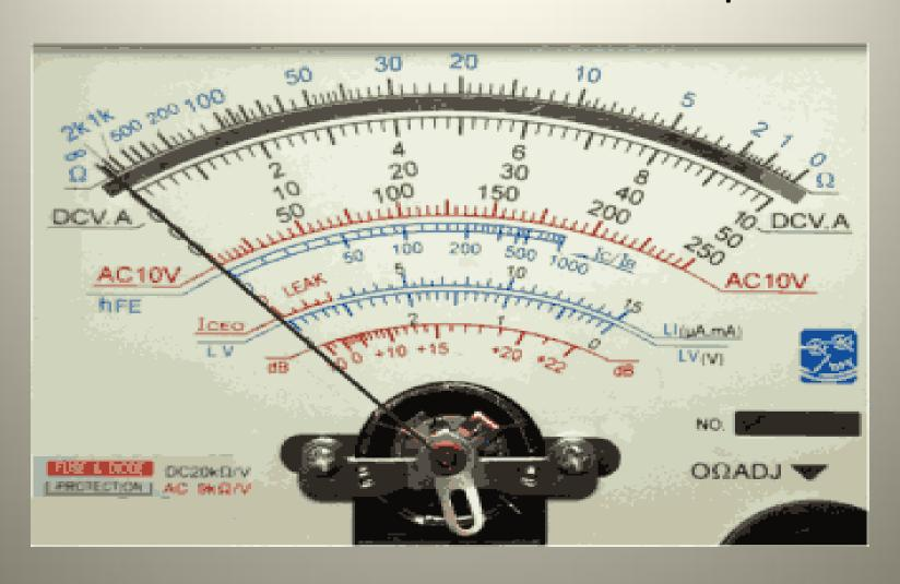
The meter reading is most accurate if you adjust the selector switch for a reading / measurement which is mid range on the scale.
