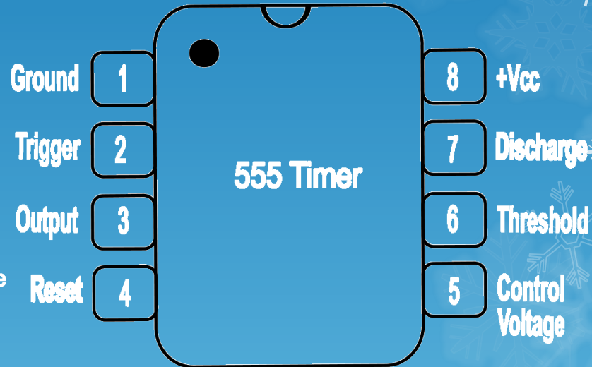
8 Pin DIP (Dual Inline Package)
